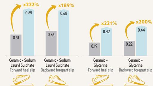
Slip resistance test according to EN ISO 20344:2021, conducted by Intertek Testing Services Shenzhen Ltd., in August 2022, on a scale of 0.0 (without slip resistance) to 1.0 (very high level of slip resistance, e.g. on dry carpeted floors). All SFC shoes are fitted with the patented, slip-resistant Shoes For Crews outsole.
